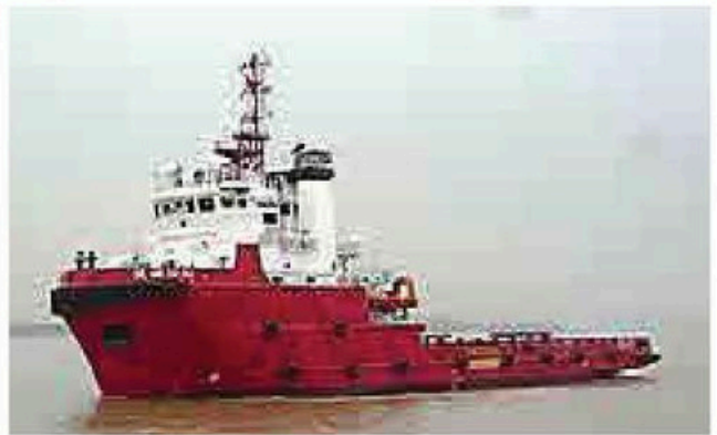
DEPU OSV, Daihatsu Propulsion Engine 6DKM-28e with Kamome CP Propeller
