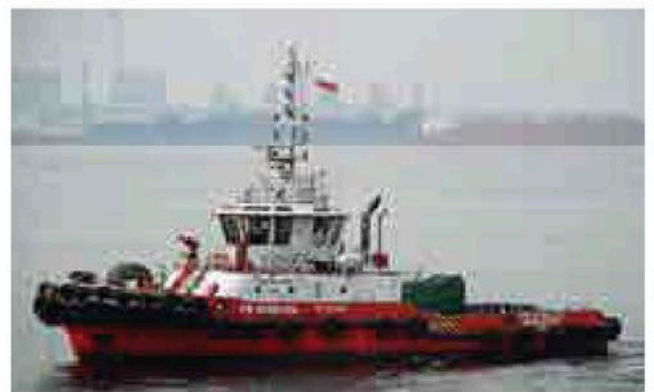
PW BERGUNIA, Daihatsu Propulsion Engine 6DKM-26e with Schottel SRP thruster
