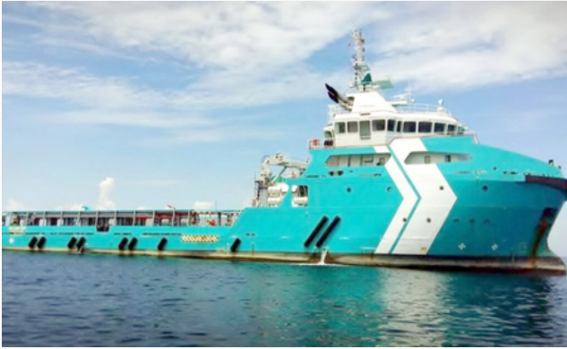
NCA80E series Diesel Electric AHTS, Daihatsu Generator 6DE-23
