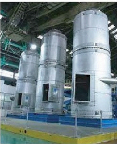
FE-made SOx scrubbers using cyclone technology
