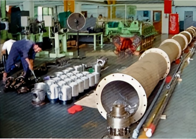
Overhauling of engine parts at the Daikai workshop
