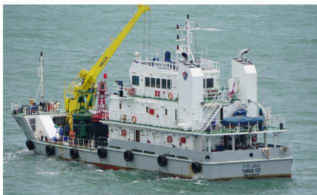
TARUA 123 Buoy Tender vessel, Daihatsu Propulsion Engine 6DKM-20e and Gearbox
