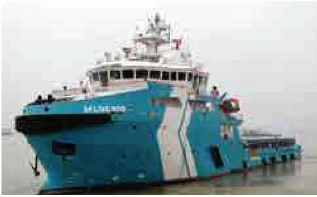
NCA80E series Diesel Electric AHTS, 6DE-23 Daihatsu Diesel generator
