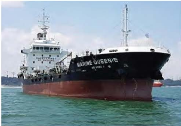
MARINE-QUEENIE, ROSE, SELENA & TINA Bunker Tanker, 6DKM-20eF(L) Daihatsu Main engine with Daihatsu gearbox
