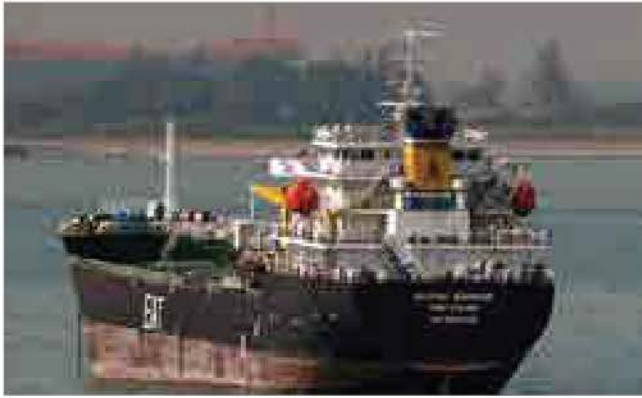
NAUTICA MAHARANI Oil Tanker, 6DKM-36 Daihatsu Main engine with Chongqing gearbox and Kamome FP propeller
