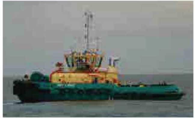
NTT-LARUT & NTT LUMUT, 6DKM-26e(F)(L) Daihatsu Main engine with Kawasaki Rexpeller and Jason FiFi
