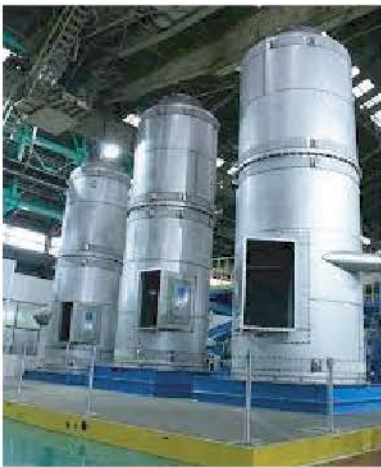
FE-made SOx scrubbers using cyclone technology
