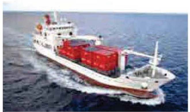
TUHAA PAE IV Cargo & Passenger vessel, 6DLM-26 Daihatsu Main engine with gearbox and Kamome FP propeller
