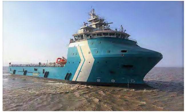
PSV-NCP4000E series Diesel Electric PSV, 6DE-23 Daihatsu Diesel generator
