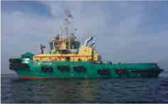
NTT-BATIK,BERCHAM,BIKAM,BERUAS, BIDOR, 8DKM-28e(F)(L) Daihatsu Main engine with Kawasaki Rexpeller and Jason FiFi
